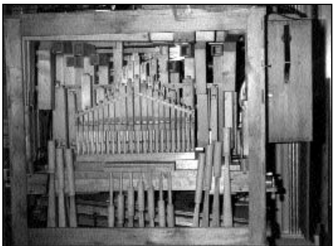
Figure 7. The later style of roll-operated style 107 Gebrueder Bruder had a case that was jammed with quality pipework. This is number 5371, with the roll box on the right side. Photo: Ron Yost.
