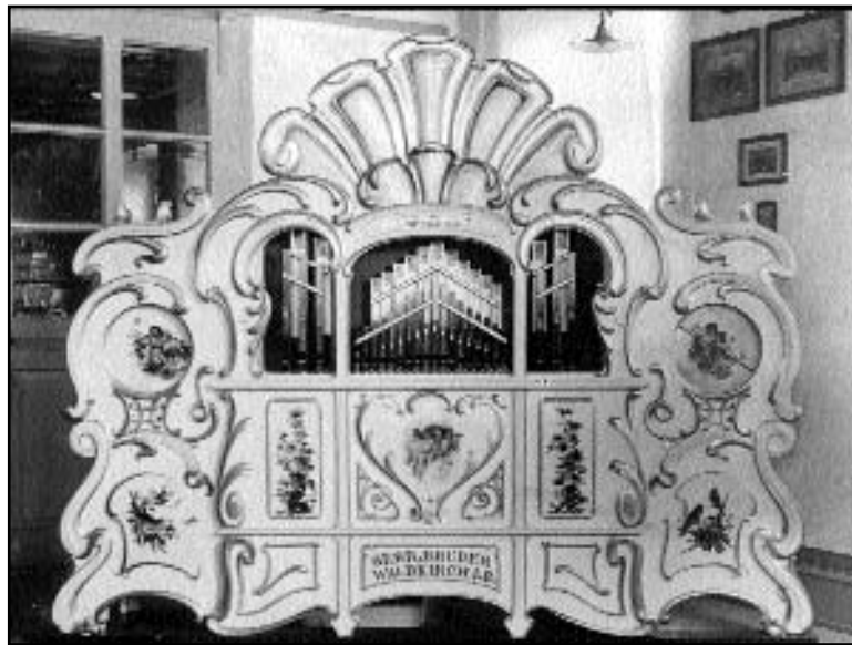
Figure 9. A rarely encountered organ is the Model 100. This factory photograph clearly shows different pipework than that found in the more common Model 107. An example of this organ exists in the U. S. Photo: Stefan Fleck.
