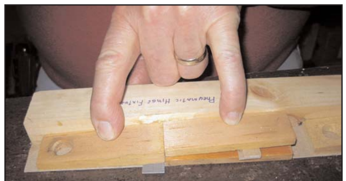
Figure 38 (below). Aligning wood blocks of secondary pneumatic.
