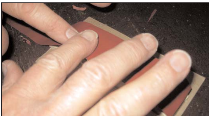
Figure 53 (above). Gasket and balance leather on secondary pneumatics.
