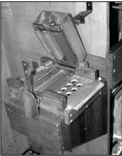
Figure 20. The restored keyframe installed in the organ.
