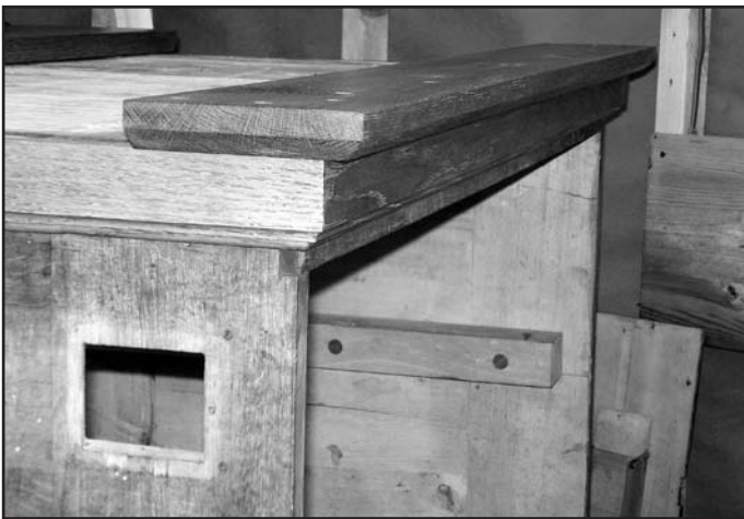
Figure 5. New sleds made for the bottom of the case.
