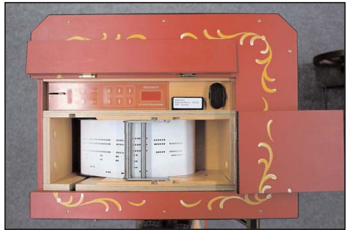
Figure 6. The barrel organs can, on request, be fitted with an integrated memory along with the music roll.
