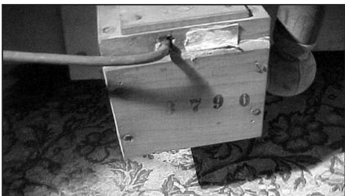
Figure 1 (above). The cut-off mechanism (mutes the organ when the end of the book has passed through the keyframe) showing the organ's serial number, 3790.
