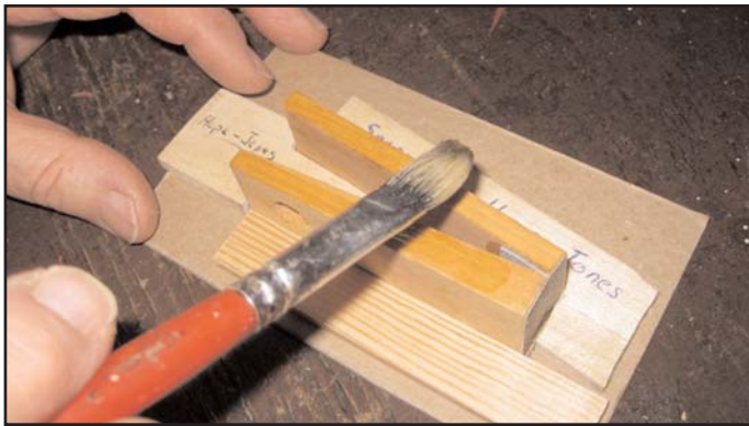
Figure 47 (above). Applying hide glue. Figure 48 (below). Applying leather. Figure 49 (bottom). Securing leather on the hinge.
