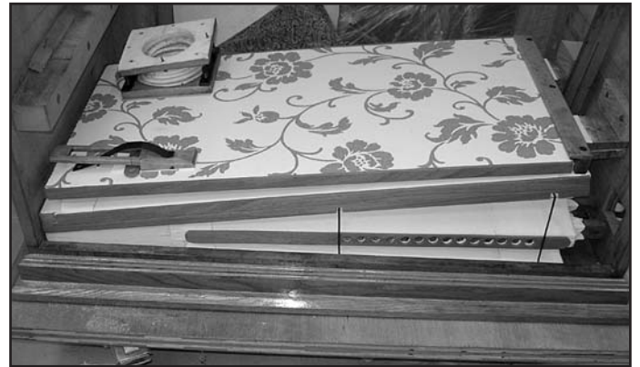
Figure 6. The completed bellows installed in the case.
