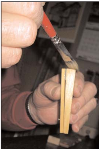
Figure 42. Applying hide glue for the outside hinge.
