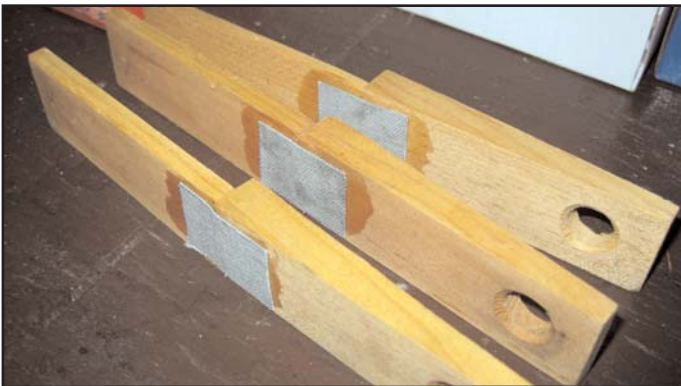
Figure 39 (top). Applying the hide glue. Figure 40 (above). Inside hinge (boat canvas) applied Figure 41 (below). Inside hinges of secondary pneumatics drying.
