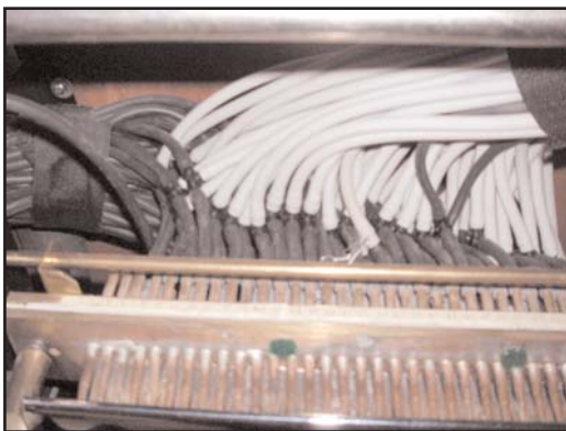
Figures 4 (above) and 5 (below). Close-ups detailing the connection from the newly installed valves to the tee behind the tracker bar.
