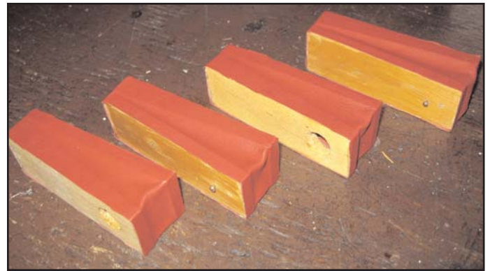
Figure 52. Re-leathered secondary pneumatics drying
