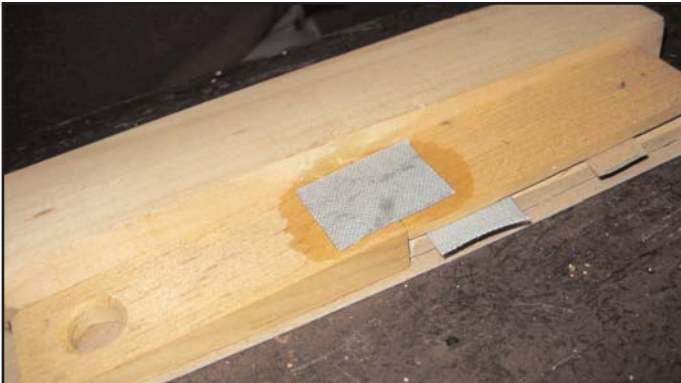
Figure 39 (top). Applying the hide glue. Figure 40 (above). Inside hinge (boat canvas) applied Figure 41 (below). Inside hinges of secondary pneumatics drying.
