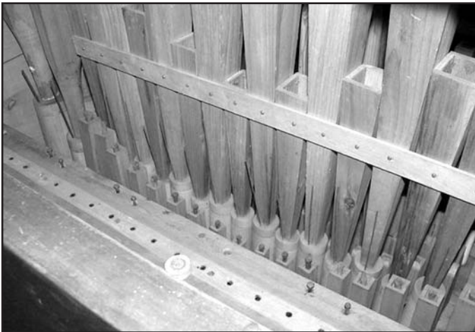
Figure 13. Trumpets prior to restoration and replacement of tuning wires and the stopped flutes. Note the condition of the stoppers.
