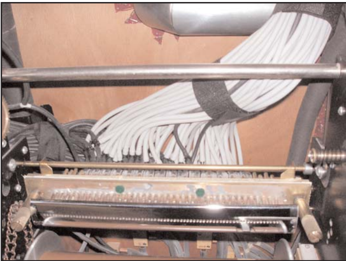
Figures 4 (above) and 5 (below). Close-ups detailing the connection from the newly installed valves to the tee behind the tracker bar.
