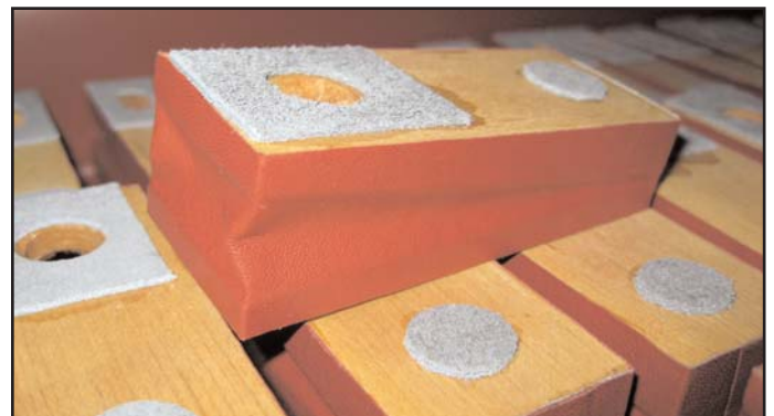
Figure 53 (above). Gasket and balance leather on secondary pneumatics.
