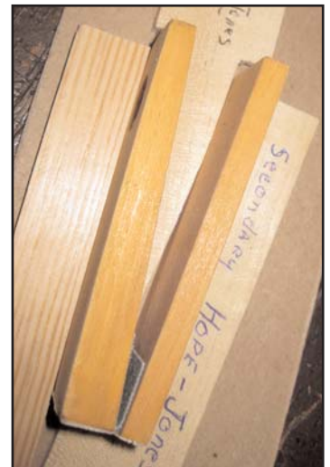
Figure 46. Secondary pneumatic placed in jig.
