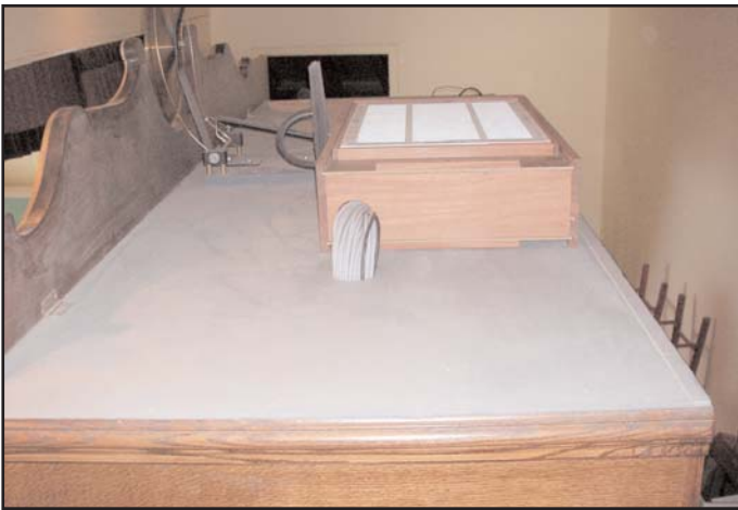
Figure 3. The valve box as it sits on top of the organ.
