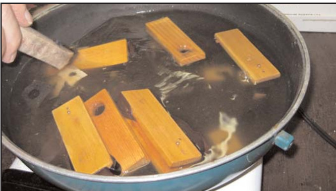
Figure 35. Removing leather, gaskets and glue from secondary pneumatics.
