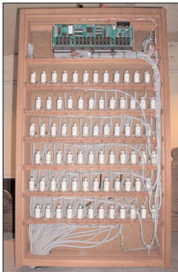
Figure 2. The box of valves for the organ.
