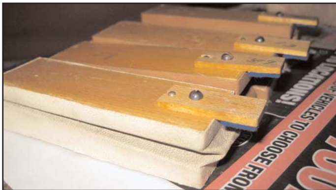
Figure 34. Secondary pneumatics prior to rebuilding.
