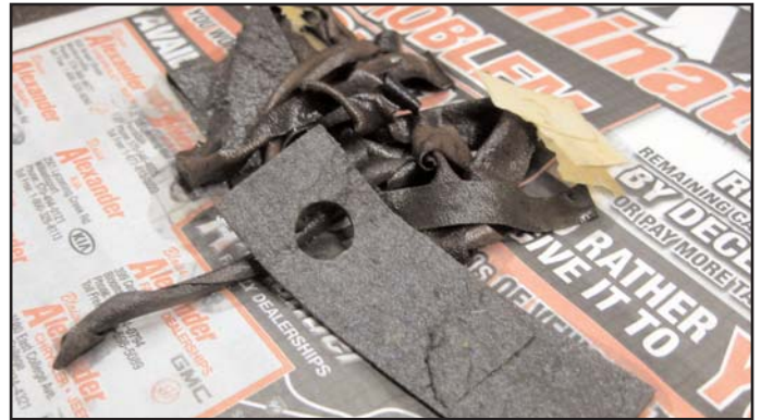
Figure 36. Leather and gaskets removed from secondary pneumatics.
